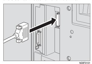
**1** Connect the other end of the SCSI interface cable to the computer.
