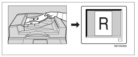
2 Adjust the guide on the document feeder (ADF) to the original size.
